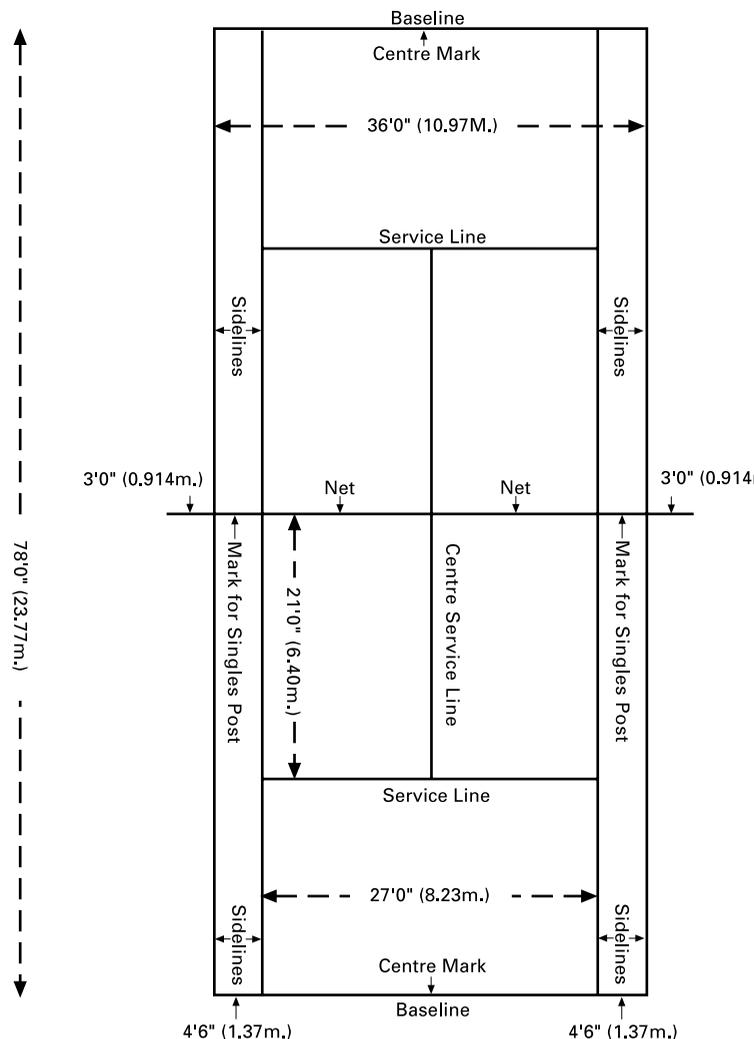
**NOTE:** All court measurements shall be made to the outside of the lines.
