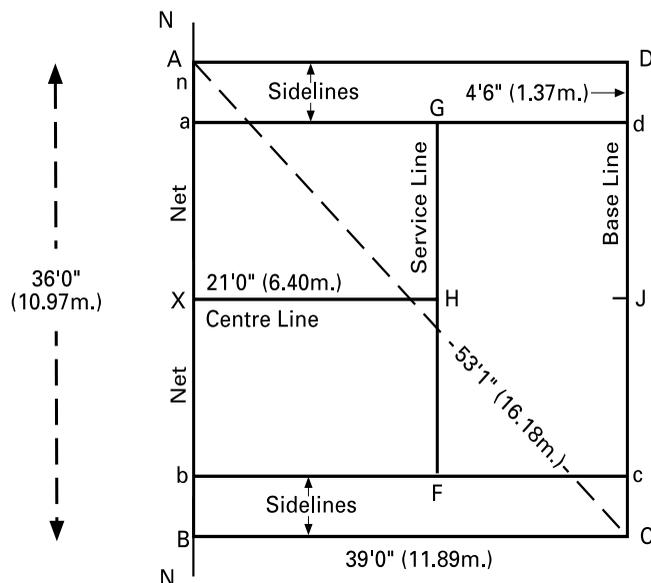
**NOTE:** All court measurements shall be made to the outside of the lines.
