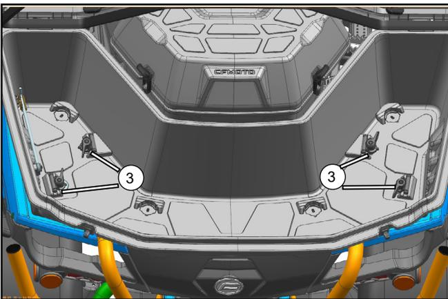
// As shown in the picture, install the four CF connect clamps (3) in the corresponding holes of the tail box, then secure the tail box by rotating the levers counter-clockwise.
