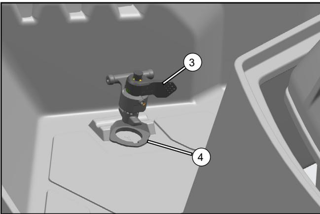
// Put the seal rings (4) and CF connect clamps (3) into the mounting hole of the tail box.
