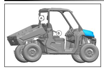
Open the cargo box (A). Remove left and right hinge mount covers (B).
