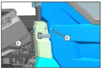
Install the bolt (D) and plastic clips (C).
