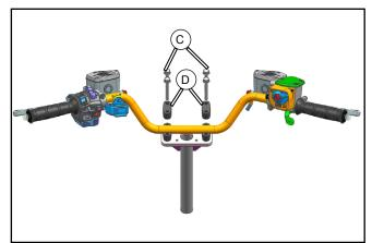
// Remove the handlebar clamp bolts (C) and clamps (D).
