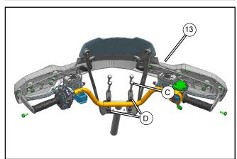
Install the windshield assembly (13) under the handlebar clamps (D). Reinstall the clamp bolts and torque evenly to specification.
