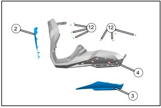
// Install right deco guard (2) and left deco guard (3) to the outside of front hand guard (4), and secure with screws (12).
