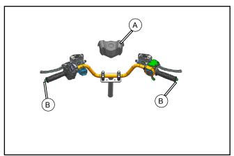
Remove the handlebar upper guard (A) and bolts (B) at both ends of the handlebar.
