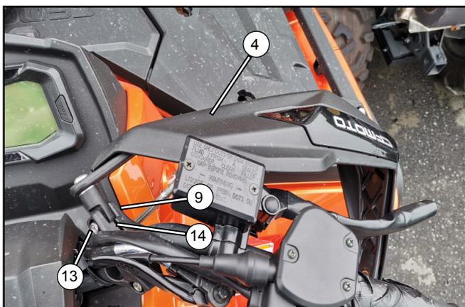
// Position the right hand guard (4) into the bracket assembly (14) as shown, then install the nut (9) and bolt (13), but do not fully tighten it.
