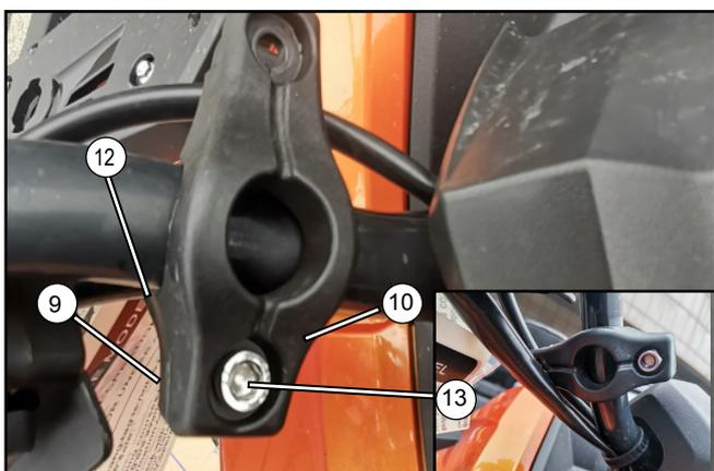
// Install bracket seat (12) and bracket press cover (10) onto right side of handlebar with nut (9) and bolt (13).
