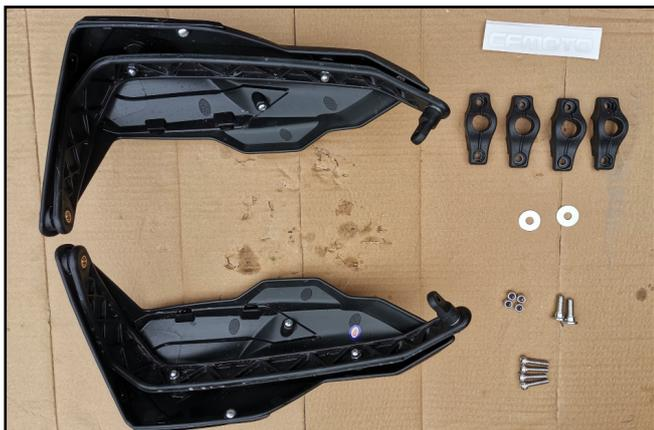
// Perform hand guard parts sub-assembly according to the diagram until it represents the completed assemblies as shown.
