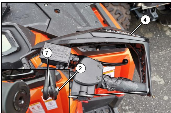
// Position the washer (7) in the middle of the end of the hand guard.
