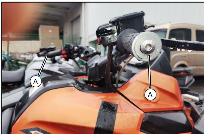
// Remove the handle bar end bolts (A).
