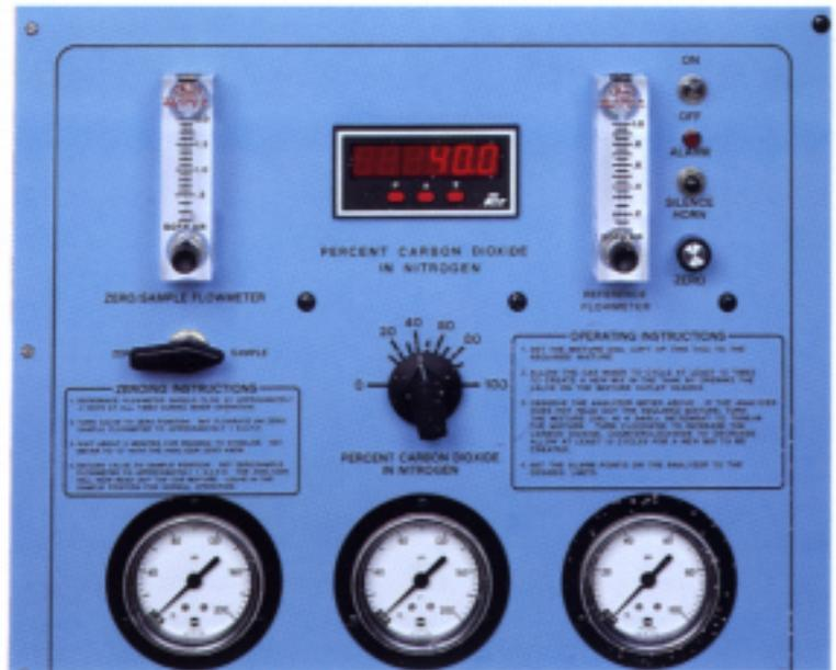
The gas analyzer built-in to the mixing system allows the operator to set the mixer to the required proportion. The gas analyzer is constantly monitoring the quality of the gas mixture.
